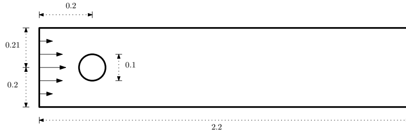
FIG. 4.4. Flow around a cylinder.
