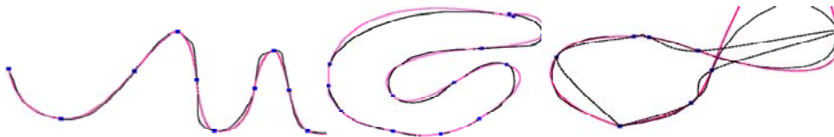
FIG. 10: Examples of curves and their reconstruction using the proposed description. Right image shows also a cardinal spline of important points.
