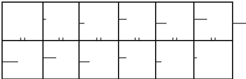
FIG. 4.3. Visualization of fluxes between mesh elements in vertical cut of the domain \Omega in time t = 2000 computed using time step \Delta t = 500 and symmetric or nonsymmetric linearization with artificial viscosity. Unitary normal component of velocity is represented by length about 35 mm.
