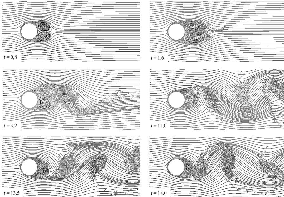
FIG. 2. Flow around the circular airfoil at  $t = 0,8$ ,  $t = 1,6$ ,  $t = 3,2$ ,  $t = 11,0$ ,  $t = 13,5$ ,  $t = 18,0$  ( $t$  - dimensionless time).
