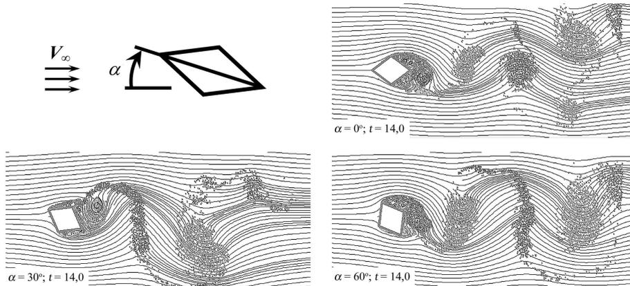
FIG. 7. Flow around the rhombic airfoil at  $\alpha = 0^\circ$ ,  $\alpha = 30^\circ$ ,  $\alpha = 60^\circ$  for  $t = 14,0$  ( $\alpha$  - angle of incidence,  $t$  - dimensionless time).
