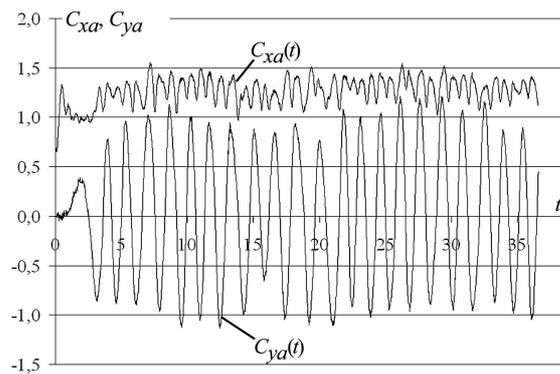
FIG. 3. Nonstationary aerodynamic coefficients for the circular airfoil. Stationary values (experimental) are  $C_{xa} \approx 1,2$ ,  $C_{ya} \approx 0$ .
