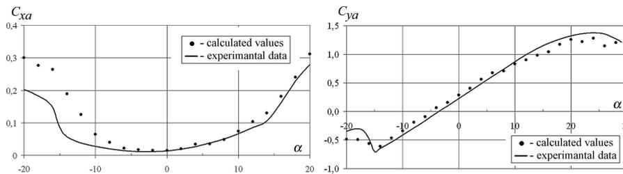
FIG. 6. Stationary aerodynamic coefficients dependencies on angle of incidence for TSAGI RII-18 wing airfoil.  $C_{xa}(\alpha)$  – drag coefficient,  $C_{ya}(\alpha)$  – lift coefficient ( $\alpha$  – angle of incidence).
