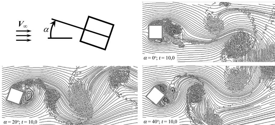
FIG. 9. Flow around the square airfoil at  $\alpha = 0^\circ$ ,  $\alpha = 20^\circ$ ,  $\alpha = 40^\circ$  for  $t = 10,0$  ( $\alpha$  – angle of incidence,  $t$  – dimensionless time).
