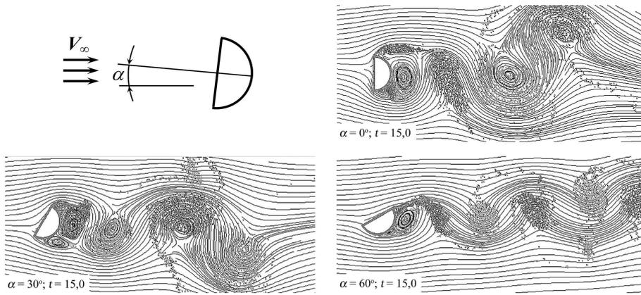
FIG. 4. Flow around the semicircular airfoil at  $\alpha = 0^\circ$ ,  $\alpha = 30^\circ$ ,  $\alpha = 60^\circ$  for  $t = 15,0$  ( $\alpha$  – angle of incidence,  $t$  – dimensionless time).
