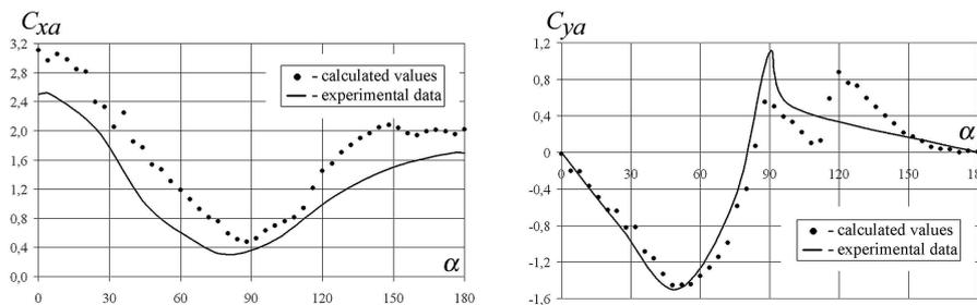
FIG. 5. Stationary aerodynamic coefficients dependencies on angle of incidence for the semicircular airfoil.  $C_{xa}(\alpha)$  – drag coefficient,  $C_{ya}(\alpha)$  – lift coefficient ( $\alpha$  – angle of incidence).
