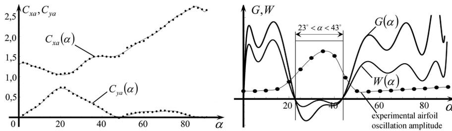
FIG. 8. Stationary aerodynamic coefficients dependencies on angle of incidence for the rhombic airfoil (left graph). Functions  $G(\alpha)$  and  $W(\alpha)$  plots for the rhombic airfoil and experimental airfoil oscillation amplitude dependence on angle of incidence (right graph).  $C_{xa}(\alpha)$  – drag coefficient,  $C_{ya}(\alpha)$  – lift coefficient ( $\alpha$  – angle of incidence).
