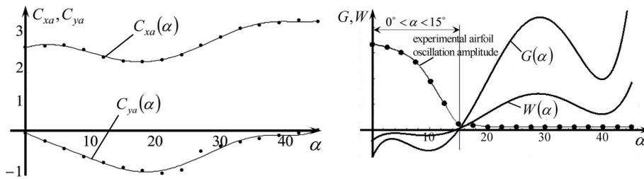
FIG. 10. Stationary aerodynamic coefficients dependencies on angle of incidence for the square airfoil (left graph). Functions  $G(\alpha)$  and  $W(\alpha)$  plots for the square airfoil and experimental airfoil oscillation amplitude dependence on angle of incidence (right graph).  $C_{xa}(\alpha)$  – drag coefficient,  $C_{ya}(\alpha)$  – lift coefficient ( $\alpha$  – angle of incidence).
