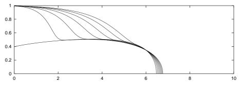
Figure 3. Subsequently saturation distribution under gravitation, after 0, 600, 1200, ..., 3600 seconds.
