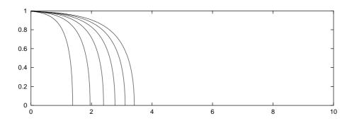
Figure 1. Saturation distribution along sand sample (of 10 cm lenghth) under gravitation, after 600, 1200, ..., 3600 seconds.
