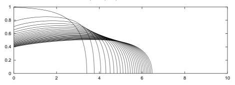
Figure 2. Subsequent saturation distribution in the sealed centrifugation, after 0, 600, 1200,  $\dots$ , 14400 seconds.
