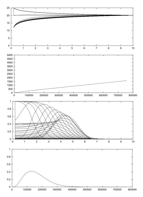
Figure 4. Simulation results of the direct problem in injection/extraction: (from top to bottom) successive profiles of hydraulic head (m) vs. radial coordinate (m); total amount of water extracted vs. time (s) during the extraction regime; successive profiles of contaminant concentration vs. radial coordinate (m); contaminant concentration at  $r = r_0$  vs. time (s) during the extraction regime.
