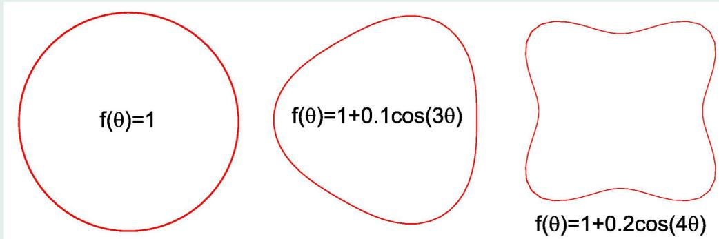
**Figure 2.1.** The Frank diagram of anisotropy.
