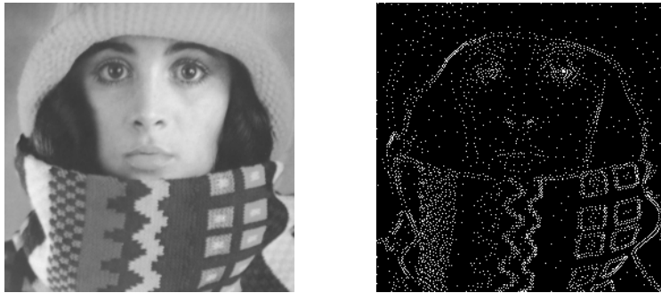
FIGURE 4.1. Left: true input image ( 256 \times 256 pixel), Right: inpainting mask with 5% density, pixel locations used for the reconstruction are marked in white.
