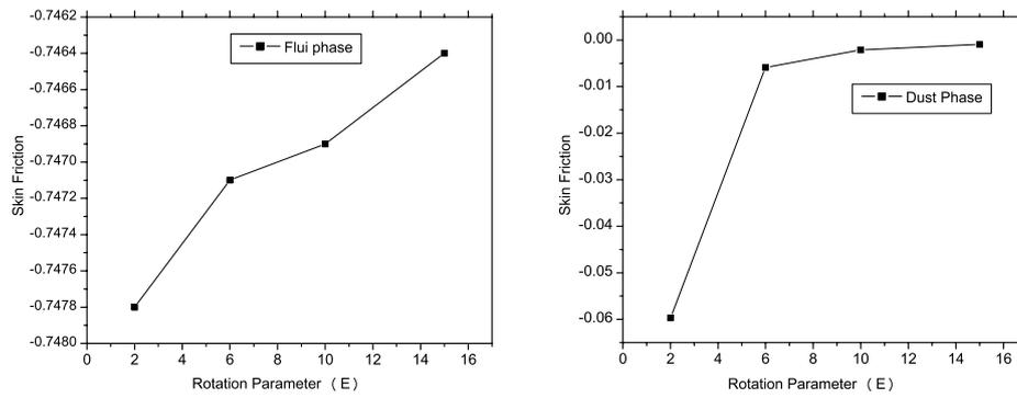
**Figure 15.** Skin friction of fluid phase and dust phase for different values of  $-E$  ( $L = 1, k = 10, l = 0.5, Gr = 5, R = 5, n\tau = \pi/4, M^2 = 5, Pr = 0.72, n = 1.0$ ).
