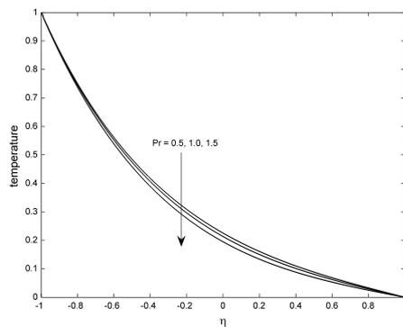
Figure 11. Variation of temperature profile for the different values of  $Pr$ .
