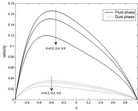
Figure 4. Variation of velocity profile for the different values of  $k^+$ .
