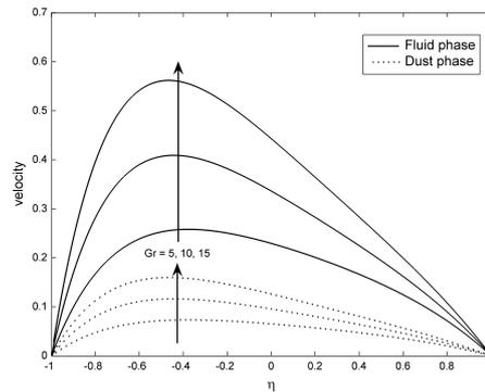
Figure 6. Variation of velocity profile for the different values of  $Gr$ .
