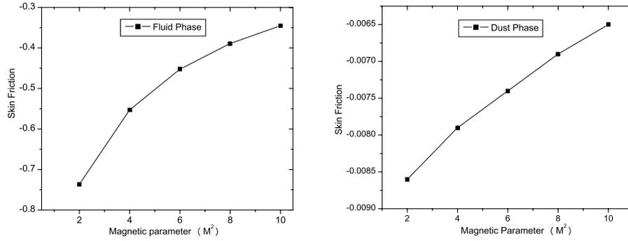
**Figure 14.** Skin friction of fluid phase and dust phase for different values of  $M^2$  ( $L = 1, k = 10, l = 0.5, Gr = 5, R = 5, n\tau = \pi/4, E = 10, Pr = 0.72, n = 1.0$ ).
