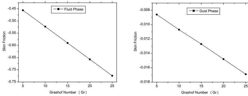
**Figure 16.** Skin friction of fluid phase and dust phase for different values of  $-Gr$  ( $L = 1, k = 10, l = 0.5, M^2 = 5, R = 5, n\tau = \pi/4, E = 10, Pr = 0.72, n = 1.0$ ).
