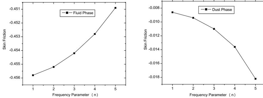
**Figure 17.** Skin friction of fluid phase and dust phase for different values of  $n$  ( $L = 1, k = 10, l = 0.5, Gr = 5, R = 5, n\tau = \pi/4, E = 10, Pr = 0.72, M^2 = 5$ ).
