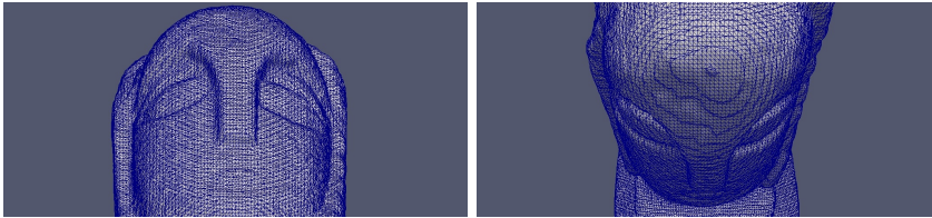
Fig. 4.4: Details of the sealer with triangulated surface.
