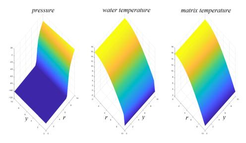
FIG. 2.1. Water pressure h and temperatures  $T_w, T_m$  in cylinder at t = 60s
