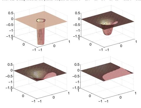
Fig. 4.3. Decay towards the planar surface at times t = 0, t = 0.002, t = 0.005 and t = 1.
