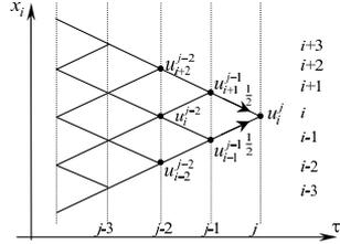
A binomial tree as an illustration of the algorithm for solving a parabolic equation by an explicit method with  $2\gamma = \sigma^2 k/h^2 = 1$ .
