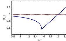
Graph of the spectral norm of the iteration operator  $\|\mathbf{T}_\omega\|$  as a function of the relaxation parameter  $\omega$ .
