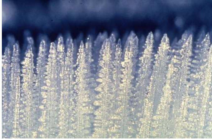
Figure 1.6: An example of a typical microstructure of an interface between mushy layer and the liquid phase. The example corresponds to the aqueous solution of ammonium chloride ( \text{NH}_4\text{Cl} ). The solid dendrites are composed of pure \text{NH}_4\text{Cl} . The horizontal length of depicted portion of the mush is 8 \times 10^{-3} m, with a typical inter-dendritic length equal to 3 \times 10^{-4} m. Source: Huppert (1990).
